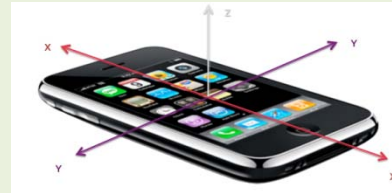
Figure 3: diagram of iPhone and its accelerometer axes
