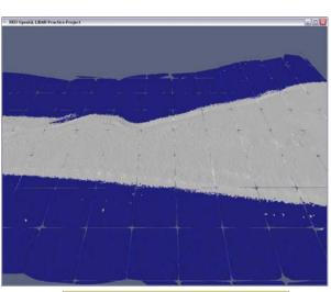
Figure 3: 3D processed LIDAR data with water and land shaded different colors
