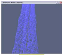
Figure 4: Triangulation of LIDAR data
